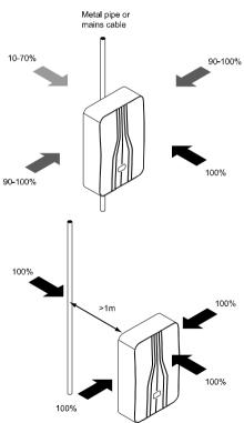
Also, If using remote aerials, never run the cable to the aerial in parallel with water pipes or other cabling unless they are more than 1m away. If you have to cross such obstacles, cross at 90 degrees.
