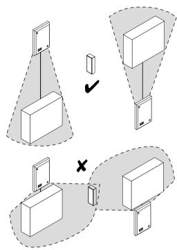
The same problem is caused by any metal box, for example a mains supply consumer unit, or water cylinder. Never mount transmitters or receivers directly below large metal objects.
